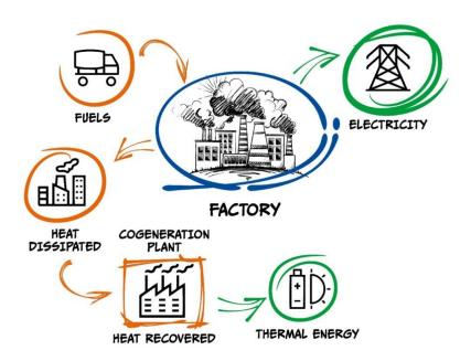
The system can self-produce 50% of the electrical energy needed by the three manufacturing plants. The equipment also provides thermal energy in the form of combustion fumes, which are recovered for the functioning of the spray driers in the ceramic body preparation unit. The new system allows a greater adaptation to the variability of electrical loads, optimizing the electrical production to the level of self-consumption of the factory and ensuring maximum heat recovery on the spray driers.
