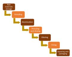
The required composition of raw materials, including also recycled wastes, is mixed and grinded in mills, either in a wet or a dry process.
