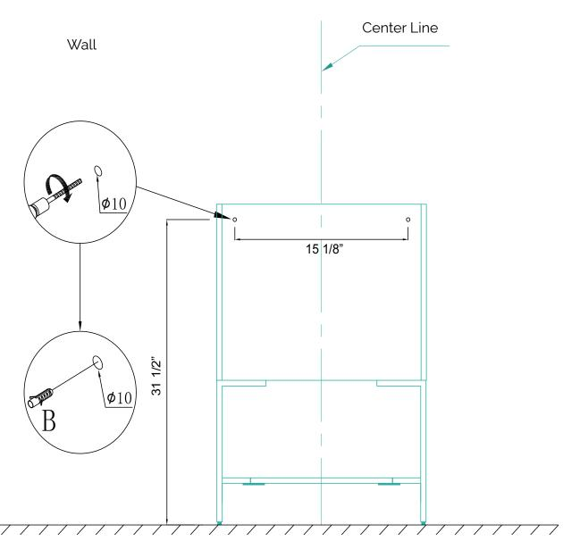
Dimensions may vary by up to 3/8". It is highly recommended to pull all dimensions of actual model for installation and measuring purposes.
