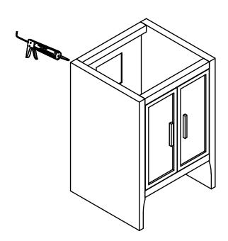
Apply caulk around the perimeter where the basin meets the countertop. Wait 24 hours for the caulk to dry fully.  Apply caulk to the perimeter of the top of the cabinet.
