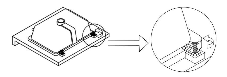
• Place and tighten the screws in the aligned holes.
